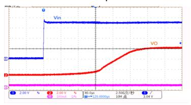
$V_{IN}$  = 7V,  $C_{IN}$  = 1 $\mu F,\,C_{OUT}$  = 1 $\mu F$  , Load = NA
