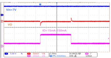
$V_{\text{IN}} = 7V, \ C_{\text{IN}} = 1 \mu F, \ C_{\text{OUT}} = 1 \mu F$
