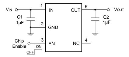
NOTE: The EN pin can not be suspended.
